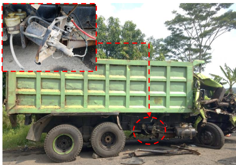
Gambar 3. Selang minyak rem putus, selang master silinder patah
