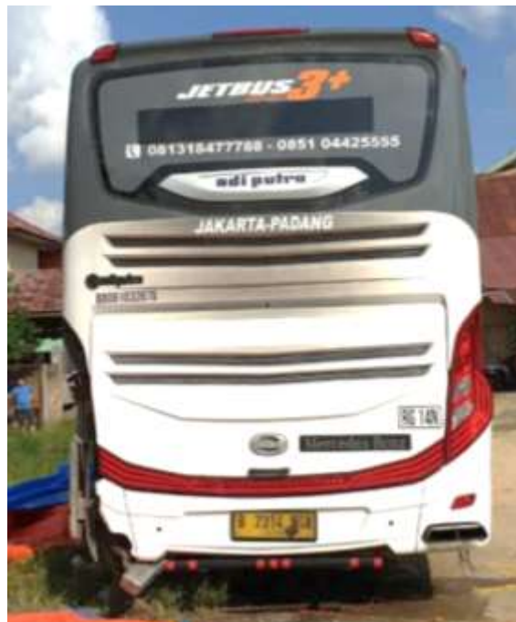
Gambar 5. Tampak belakang mobil bus lensa lampu kiri pecah
