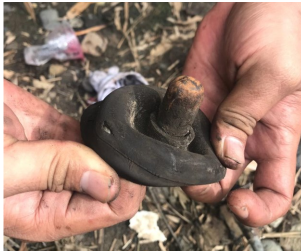
Gambar 6. Seal Cylinder rem roda belakang kiri robek
