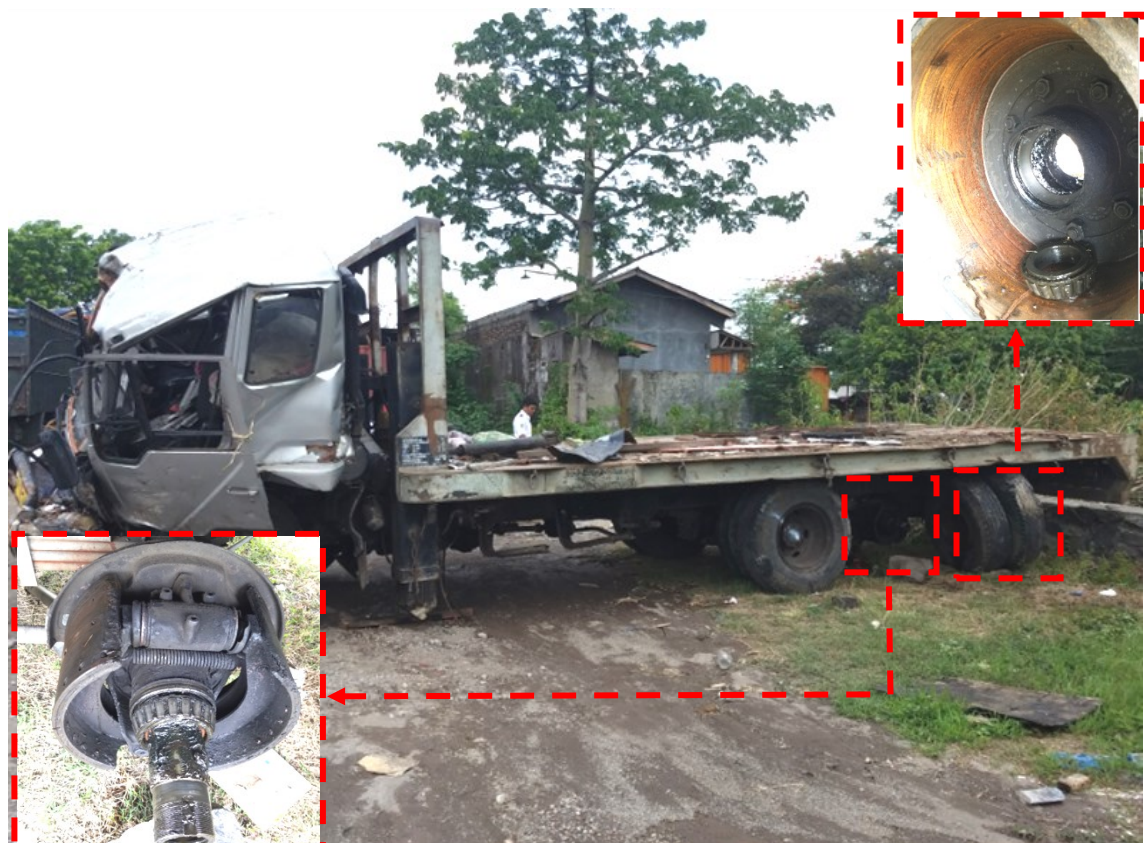
Gambar 6. Seal roda sumbu ketiga getas dan pecah (bocor grease), tebal kampas rem sejajar paku keling dan seal silinder roda rem sobek
