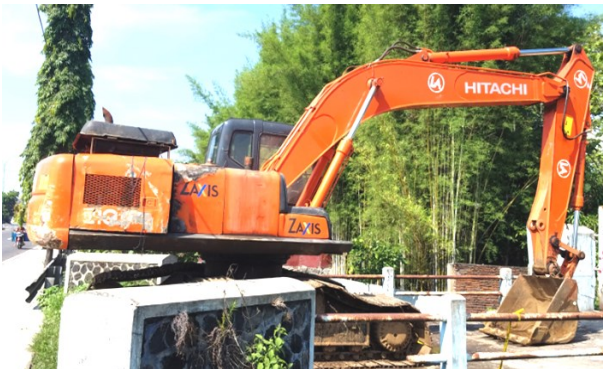
Gambar 15. Excavator muatan truk flat deck
