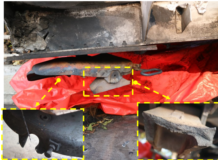
Gambar 20. Fifth Wheel Truk Trailer Tangki Patah
