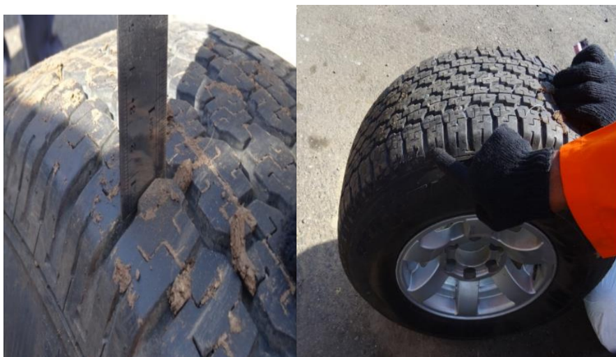
Gambar 2. Ketebalan Telapak Ban 6-7 mm.
