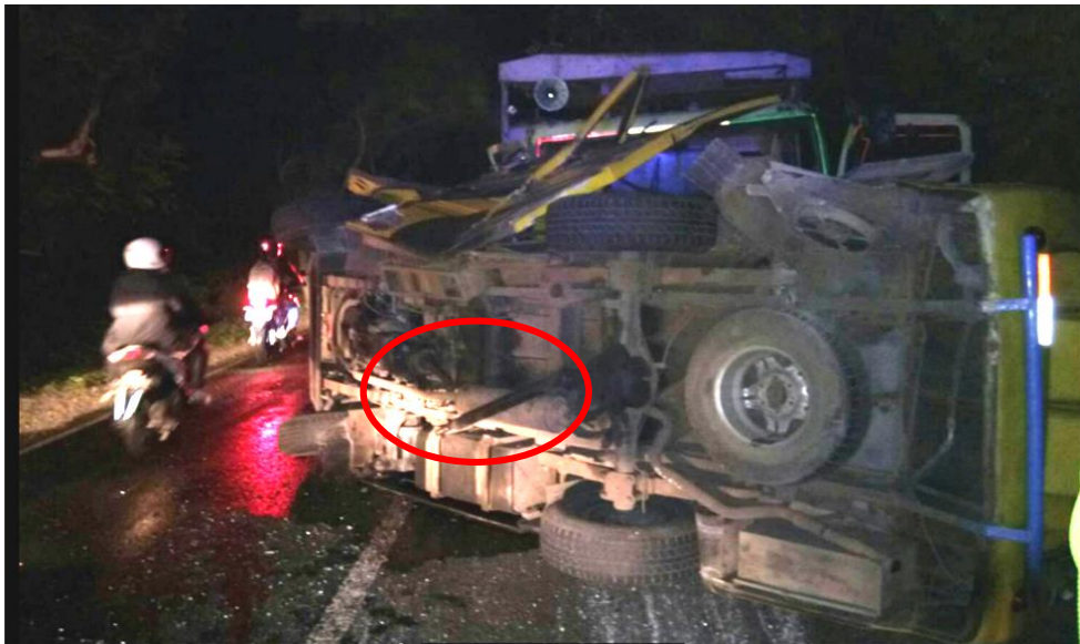
Gambar 9. Propeller shaft patah
