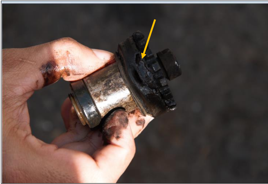
Gambar 6. Karet seal silinder rem sumbu depan kiri sobek
