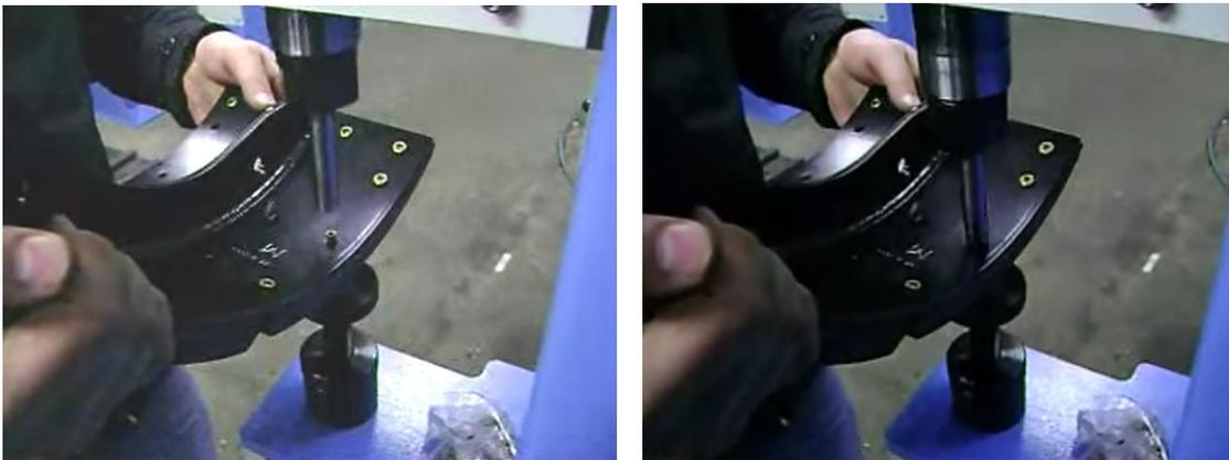
Gambar 63. Peralatan riveting semi otomatis tanpa *loader* paku keling.
