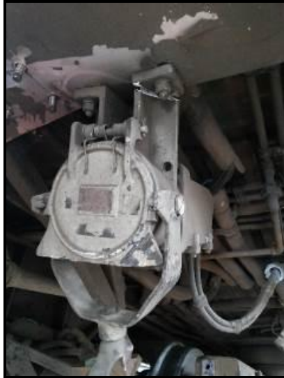
Gambar 14. Adaptor coupler electric rusak
