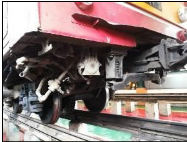
Gambar 6. Cow hanger rusak parah
