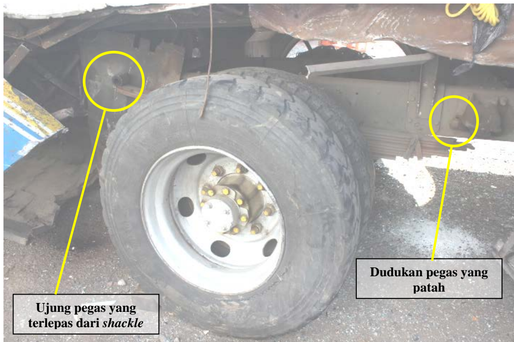
Gambar 12. Suspensi roda kanan-belakang Mobil Bus AD-1543-CF
