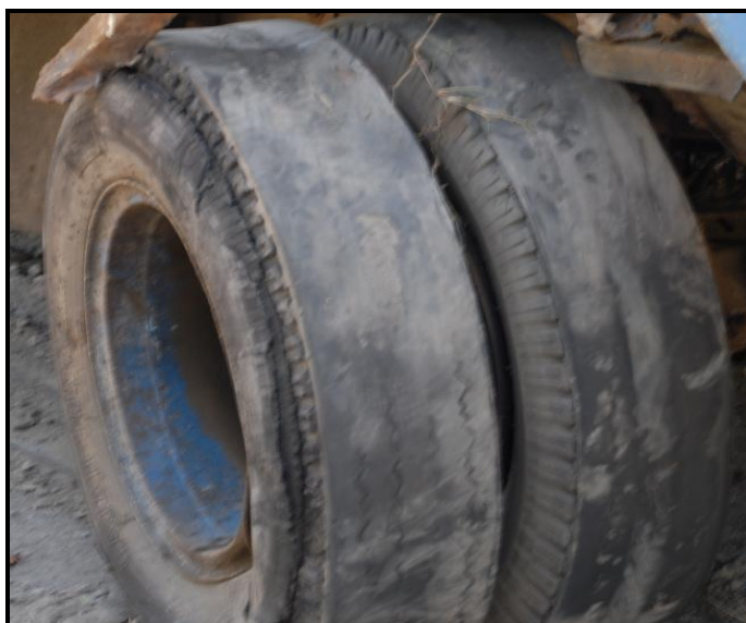
Gambar 3. Ban belakang mobil bus AD 1444 BE gundul
